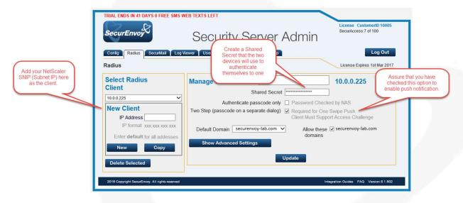
Communication will RADIUS and is expected to be operating on the standard TCP Port 1812. The SecurEnvoy SecurAccess Server is the RADIUS host.
